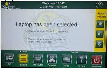
Plug the supplied HDMI and USB cables (on top of the podium) into the laptop. Then press the button labeled 'LAPTOP' on the switch device on the podium.
